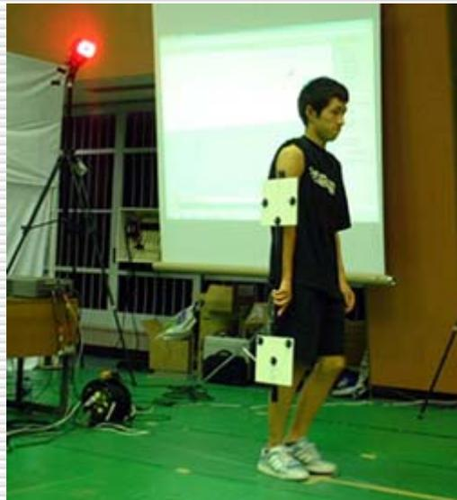
2. The subject walked on the walkway illustrated in Fig. 1, holding a bar shown in Fig. 2, as a manner shown in Fig. 3. The accuracy of the systems were tested by comparing the true value and measured value of the distance between the two markers attached at the both ends of the bar. The results are shown in Table 1.
